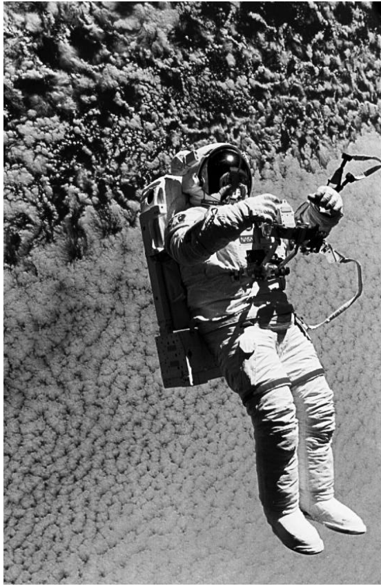
Mark C. Lee test flies the Simplified Aid for Extravehicular activity Rescue (SAFER) device during the STS-64 mission.
