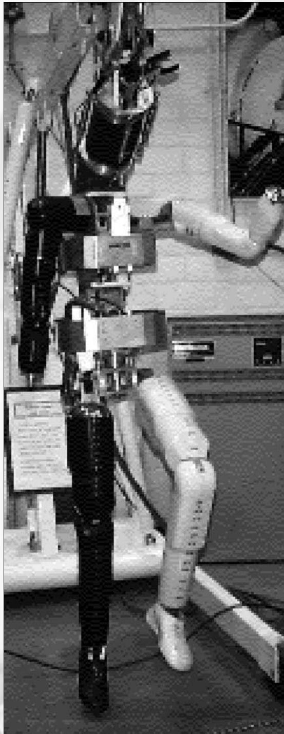
Spacesuit Robot The forces required to move suit arms and legs when the suit is pressurized are measured with this specialized robot. The robot is placed inside a suit. A gasket seals the neck of the suit. The suit is then pressurized through the robot's "head." Joints in the arm and leg of the black side of the robot are bent on command and the forces are measured. The white side of the robot is non-functioning. Only one side of the robot is needed for data and the white side serves only as balance.
