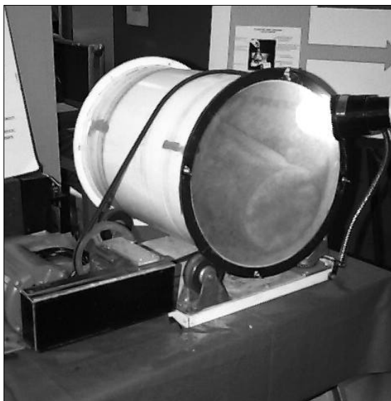
Fabric abrasion tester in use at the NASA Johnson Space Center. The white drum contains an inflated cylinder made from the outer fabric of a spacesuit. The drum also contains lunar sediment simulant. An electric motor with a pulley drives the drum.
