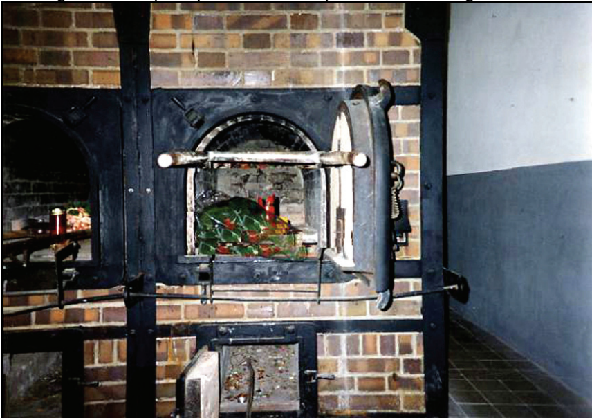
Document 46a: Crematorium of Mauthausen. Topf coke-fired double-muffle oven Auschwitz type. (Cf. document 43). Photo composition showing how high the stretcher would have had to be raised for it to be introduced into the chamber above the first two superimposed corpses.
