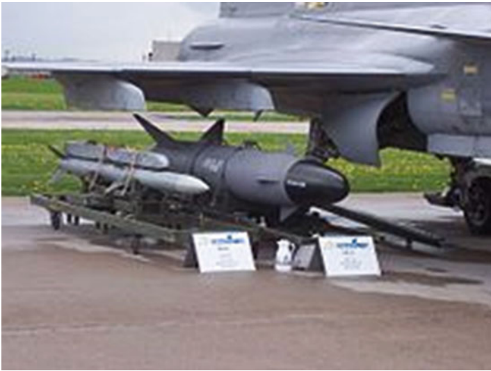
Fig. A.18 RBS-15F Anti-Ship Missile (on right) under the wing of a JAS 39 Gripen Fighter
