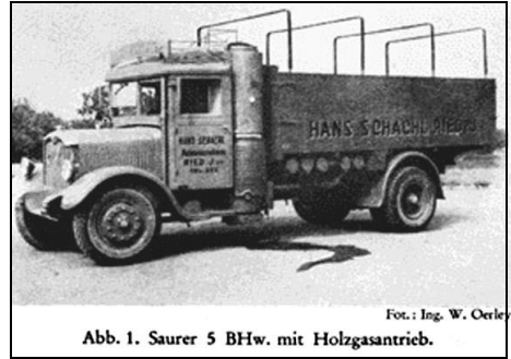
Abb. 1. Saurer 5 BHW. mit Holzgasantrieb. Illustration 4: Another German war-time producer gas truck form Saurer (Type 5 BHW)
