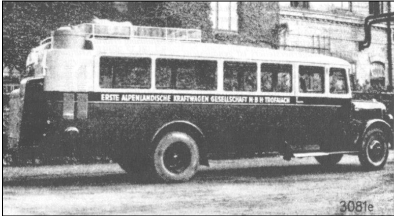
Illustration 1: A typical gas wagon which had originally been a conventional bus but which was subsequently retro-fitted with a gas-generator and a Saurer engine. 125
